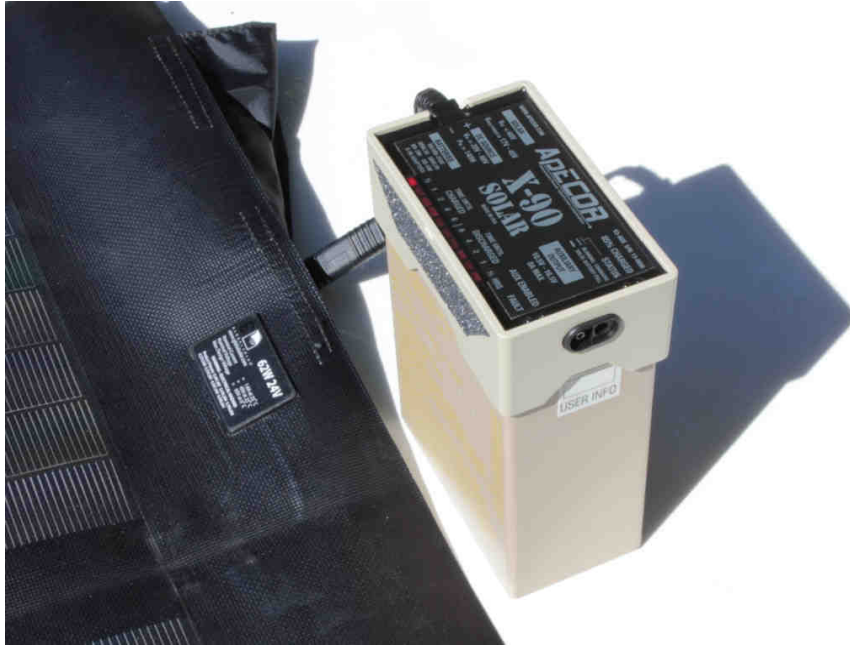
Figure 2: X-90 charging a BB-2590/U using the Global Solar P3-62W/24V panel
