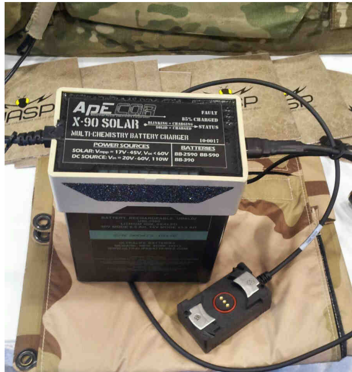
Figure 5: X-90 Charging a BB-2590/U with an extension cable, auxiliary output powering a PRC-148/152 battery eliminator adapter
