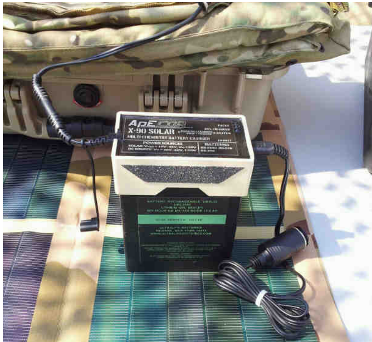
Figure 3: X-90 Charging a BB-2590/U from a DC Source, with a 12V CLA adapter output
