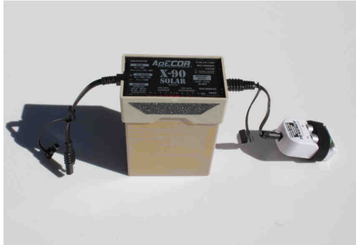
Figure 4: X-90 Powering a RCR-123A LiFePO4 battery charger
