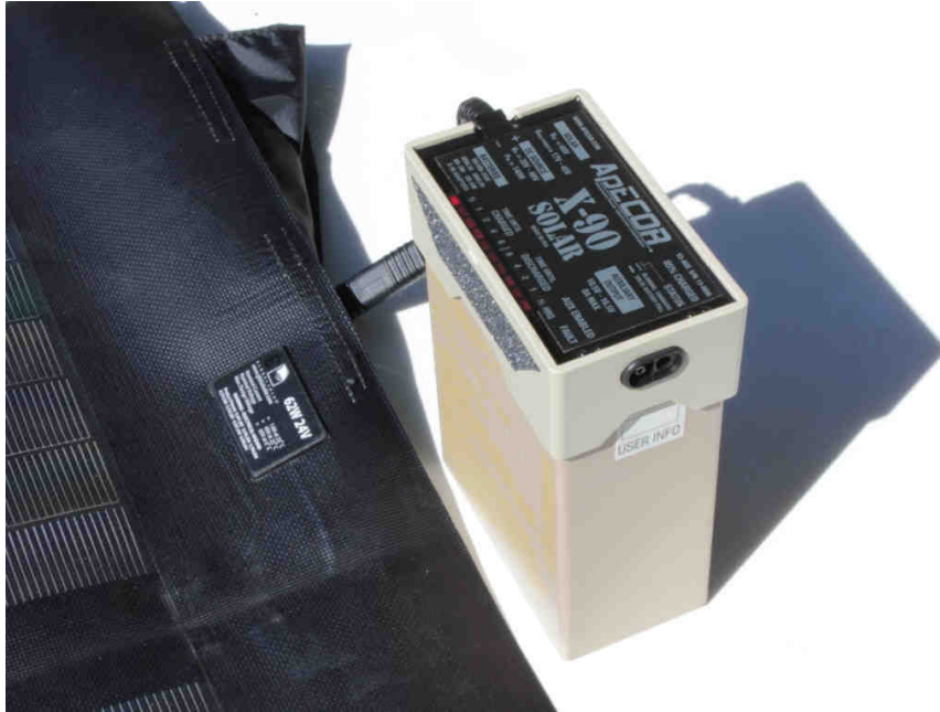
Figure 2: X-90 charging a BB-2590/U using the Global Solar P3-62W/24V panel (X-90 V3 AUX shown)
